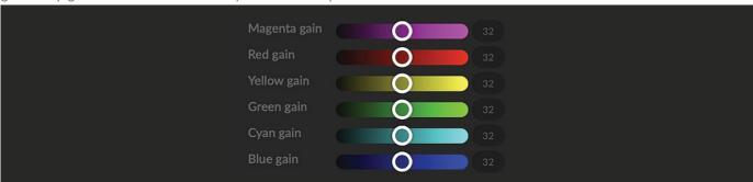
By increasing the gain value, the camera will add additional intensity to all parts of the image pertaining to this colour. For example, if you increase the Red gain value to 64 all pixels that are red in the image will have a boost of colour compared to other colours in the image resulting in a more vivid representation of this colour.
