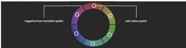
In P100 Colour Matrix controls you can adjust the colour offset in a negative (counter clockwise) or positive (clockwise) direction, effectively moving the cameras response to any colour towards its neighbouring colour transition point.
