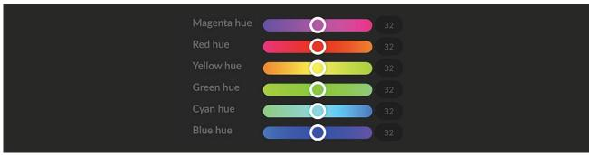
Adjusting individual colour Hue can assist dramatically in matching colour representation from the camera to true-to like colours or matching the P100 to other cameras in your production.
